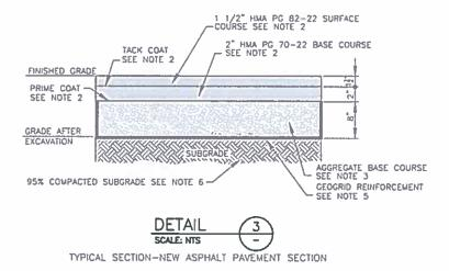
For the Hotel Wharf Asphalt pavement, shows 2" and 1.5" thick layers. We would like to confirm if it's acceptable to place 2" and 1.5" thick of same job mix (binder course with AR16000). Please confirm this is acceptable.
