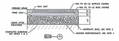
For the Route 11 Asphalt pavement in drawing as above, shows 1.5" thick in two layers. We would like to confirm if it's acceptable to place Asphalt 3" thick (Binder Course with AR16000) in one layer instead of 1.5" x 2 layers. Please confirm this is acceptable.
